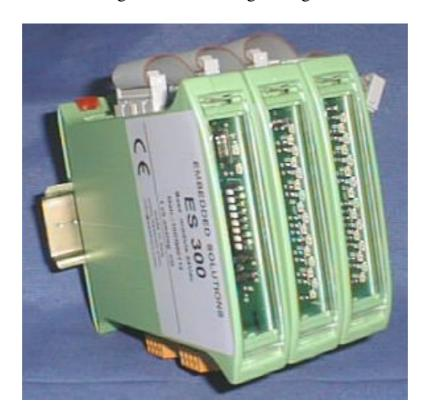
This device is particularly suitable for machines with a rotating part, where the I/O signals of the control panel can be replicated in the rotating part simply using a two-ways slip ring.
